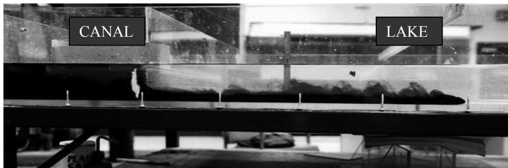
Figure 2 Profile view of the saltwater plume entering the lake; \Delta_{\text{sal}}=6 ppt; \Delta T=0^\circ\text{C} ; sill at 1/3 of lake depth
