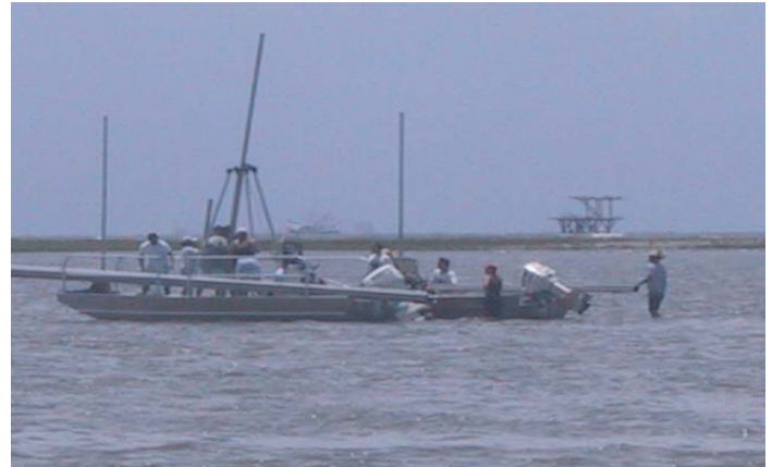
UNO students acquiring vibracores in Timbalier Bay, Louisiana from the R/V Mudlump and Greenhead. Cores were used to map the distribution of subsurface paleo shorelines that contain sandy strata suitable for coastal renourishment projects.
